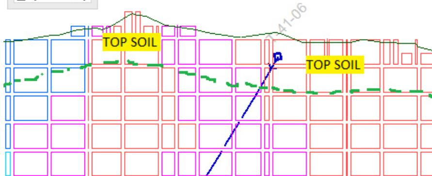
Dwg.4. Vertical section of RESMODEL. 10.7m thick top soil shows AU 2.6 g/t in the RESMODEL cells in close vicinity of the hole trace while the drill hole logs indicate top soil with the subgrade ore -- 0.2 g/t.
